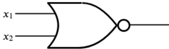
$$f = x_1 \downarrow x_2 = \overline{x_1 + x_2} = \bar{x}_1 \bar{x}_2$$
